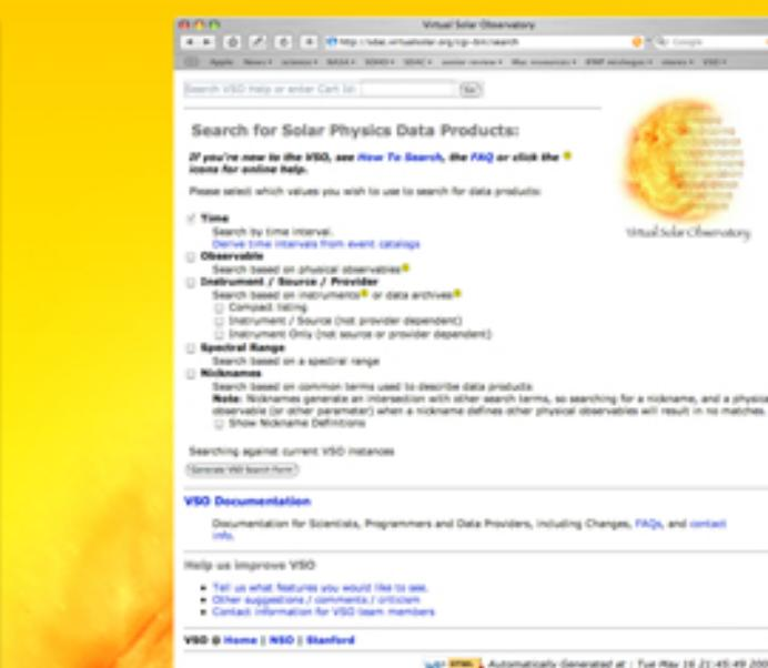
**A search starts simply enough:** All VSO searches are based on a time range and some combination of other parameters (physical observables, instrument, data provider, spectral range, or combinations of these known as “nicknames” (e.g. “EUV image,” “vector magnetogram”).
